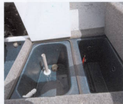
The live bait tank and anchor well are well positioned and come as standard.
